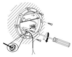
Terminate the cable into the terminal block (See section 5. Connection Diagram)
