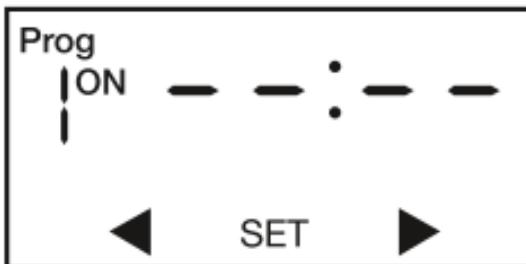
Use 'Temp' or 'Mode' to set the time, using 'Prog' to change between hours and minutes.
