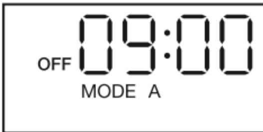
In both auto, and timed mode, the ON OFF will reflect the output of the TRT05.
