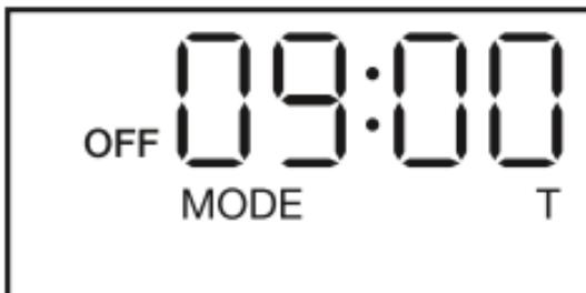
In operating mode, if 'Temp' is pressed briefly, the display changes to show the actual room temperature (not the set temperature).
