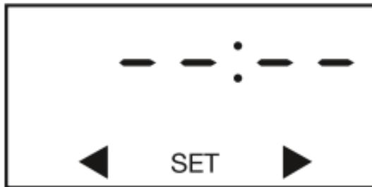
Use 'Temp' or 'Mode' to set the hour. 'Temp' increases the numeric value and 'Mode' decreases the numeric value. The hour is a 24hr clock.
