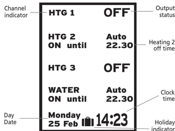
The TRT038/9 has a back lit LCD matrix display, which shows the 3/4 channel names and their status (back lighting occurs when any button is pressed). It shows the current day/date, and the current time. There is a suitcase symbol displayed if the unit is in holiday mode.
