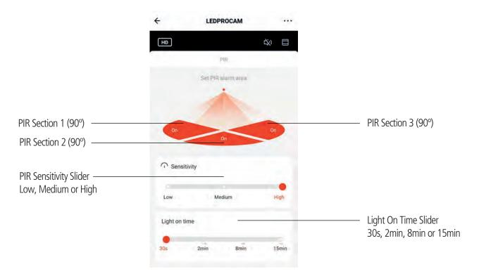
Notice the PIR detection can be combined to allow for a full 270° area of detection or as low as a 90° area of detection from the left, right or centre. You can also enable or disbale the PIR detection areas to suit your installation environment i.e. left and right areas to detect only while the central area remains disabled.
