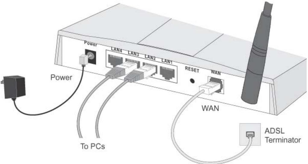
**Figure 4: Installation Diagram**
