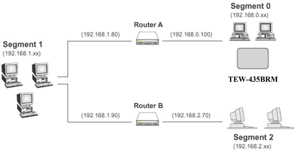
Figure 47: Routing Example
