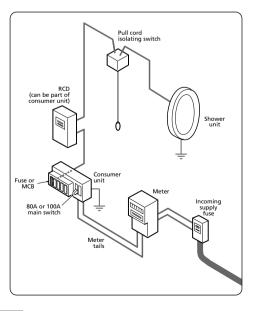
**6** For close circuit protection DO NOT use a rewireable fuse. Instead use a suitably rated miniature circuit breaker or cartridge fuse (**see table below**).
