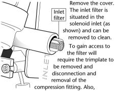
depending on the incoming pipework arrangements, if there is not enough slack in the pipework, it could mean the removal of the unit from the wall.
