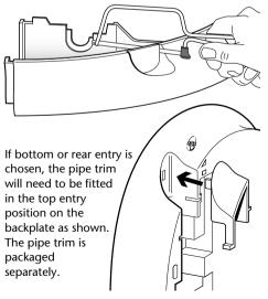
If installing a supply pipe from the rear or bottom, the centre of the inlet valve to the wall surface is 21mm.
