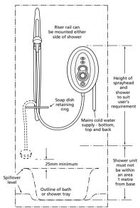
Position the unit where it will NOT be in direct contact with water from the sprayhead. Position the shower unit vertically.
