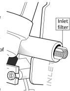
fitting. The plastic filter protrudes from the inlet so ensure it is in place before connection.
