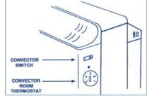
thermostat knob is marked 1 to 5. The higher the setting number chosen, the higher the level at which the room temperature will be controlled.
