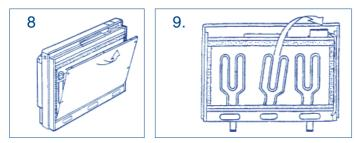
9. Remove one element to allow access for the back row of bricks. On the 724N remove the element to the right of centre, on the 718N remove the central element, on the 712N the left hand element should be removed.
