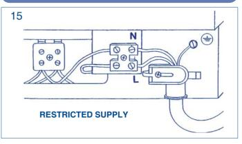
**16. Connection of supply to Convector** is through a cable clamp in the case of the front panel.
