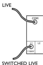
For 2 or more gangs the live wire may be connected to each COM terminal by means of a short length of sleeved wire.
