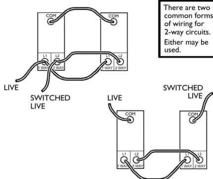
There are two common forms of wiring for 2-way circuits. Either may be used.
