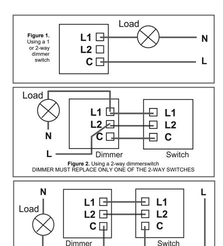
Figure 3. Using a 2-way dimmerswitch DIMMER MUST REPLACE ONLY ONE OF THE 2-WAY SWITCHES
