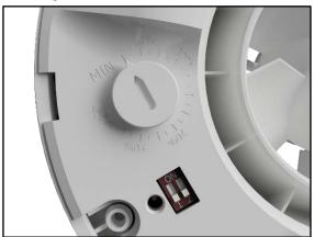
Speed can be adjusted while the fan is isolated from the mains with the inner grille removed or with the inner grille screwed on and the fan powered up. Note the fan speed is only adjustable within the first 5 minutes of mains power.
