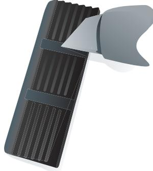
8. Install the largest cable at the bottom of the gripper slot first. Then the next size on top and the smallest last. Fit the gripper first, then each section of cable in turn to prevent the cables moving up the gripper slot.
