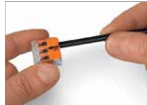
3. Lower the lever to close the clamp to complete the connection. 4. To remove, lift the lever and pull out the conductor.
