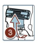
Turn the AFDD / RCBO on - Resetting the toggle allows the indication lamps to be lit
