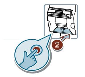
• **Reset** the light indication by pressing the T test button
