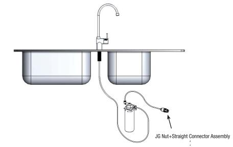
4. Align the tabs of the cartridge with the filter housing and insert it into the socket. Turn the cartridge a quarter turn to the right until it stops and locks into position.
