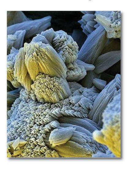
**Limescale** is the hard, off-white, chalky deposit found in kettles, hot-water boilers and the inside of inadequately maitained hot-water central heating systems. These types of limescale differ slightly due to their origins.
