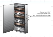
A barrier or enclosure that protects against access to live parts with wires or strips 1.0 mm thick or greater could be coded IP4X or IPXXD. IP4X also denotes protection against the ingress of solid foreign bodies 1.0 mm in diameter or greater.
