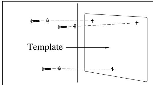
2. Install the screws (included) into the wall.
