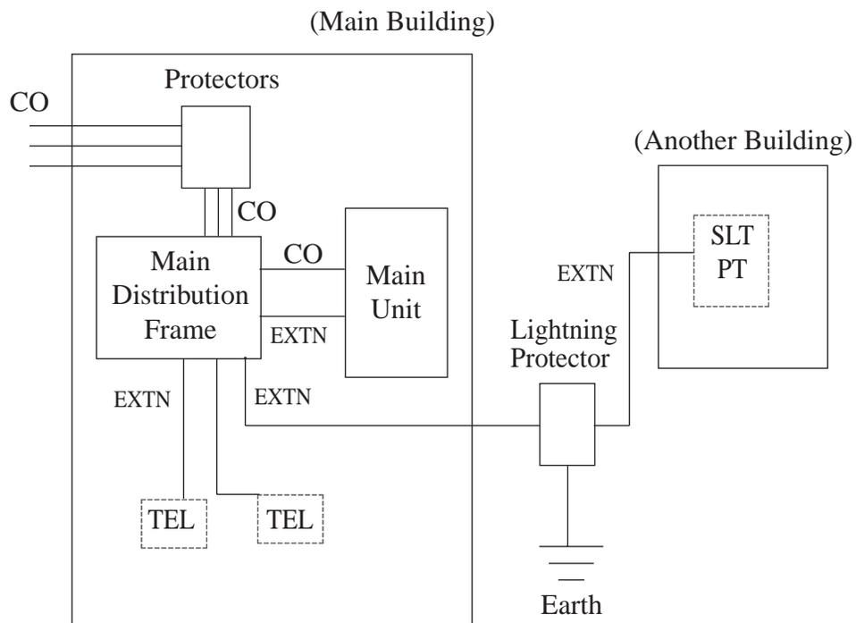
**Note** • The lightning protector for an extension is different from that for CO.
