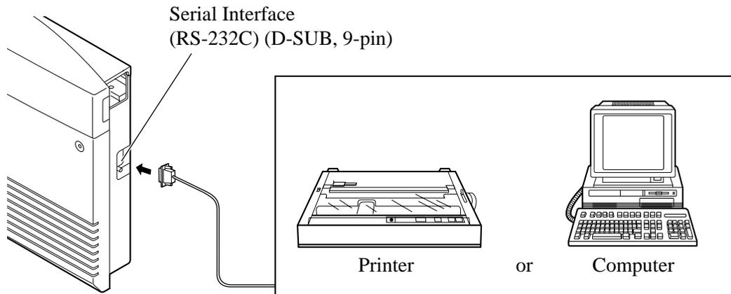
Arrange the cables so that the printer will be connected to the system as shown in the appropriate chart on the following page.
