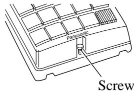
1. Loosen the screw to open the doorphone unit.
