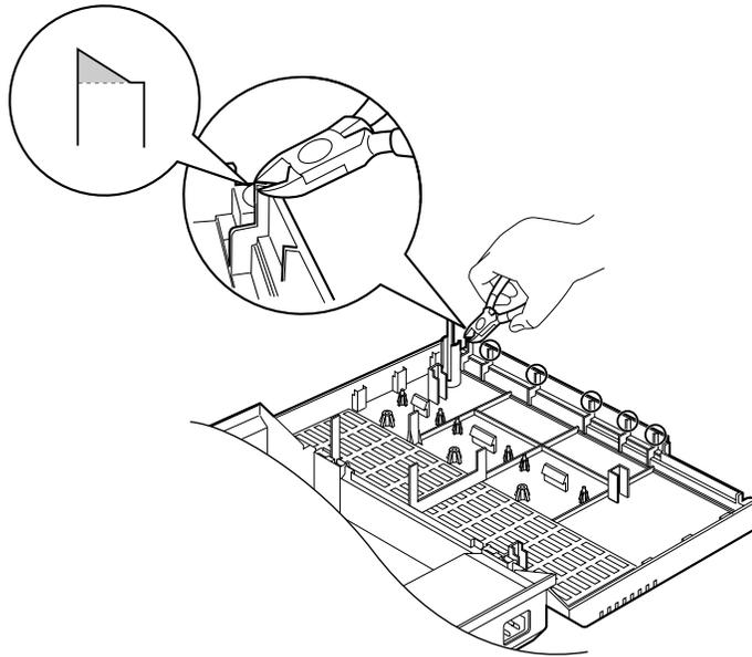
4. First, insert the plastic spacer into the hole on the KX-TA62477. Attach the 2 extension connectors to the system, install the KX-TA62477 and secure the 2 extension spacers.
