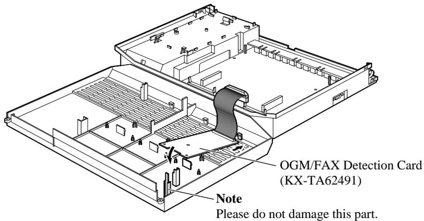
4. Insert the flat cables to the card connector.
