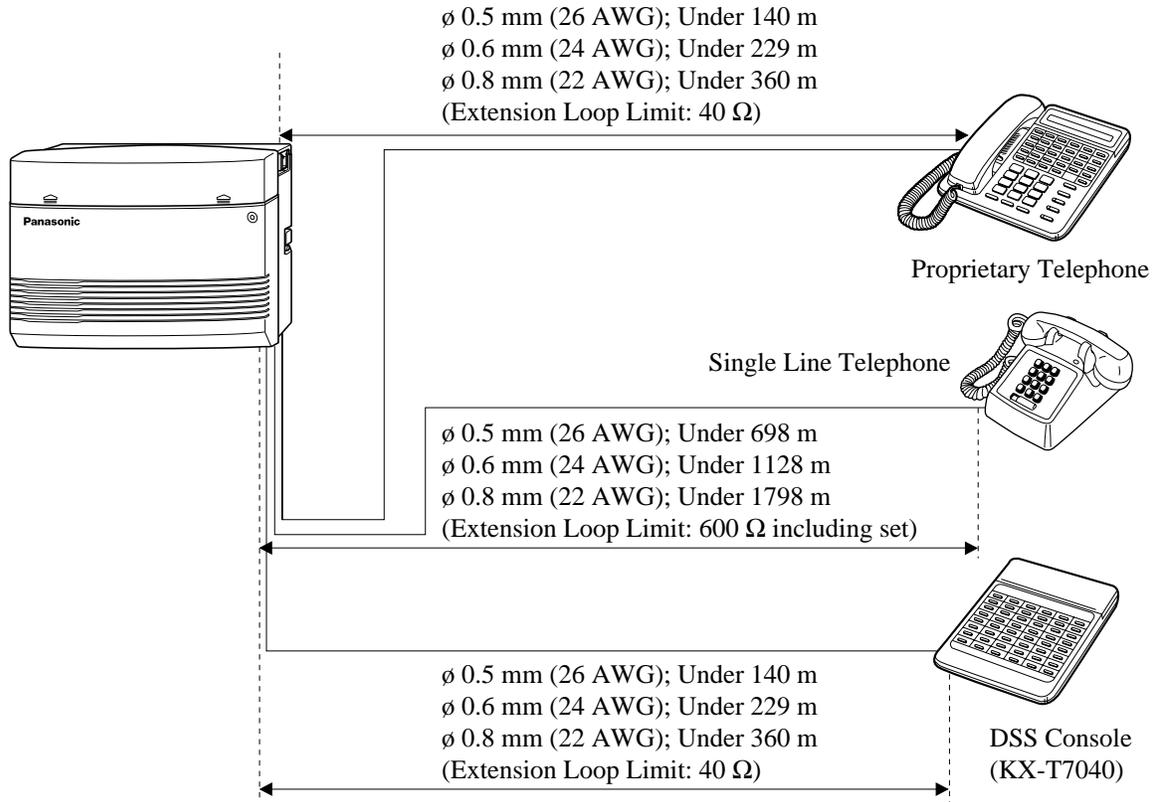
2 or 4-conductor wiring is required for each extension as listed below. There are 4 pins possible for connection: "T" (Tip), "R" (Ring), "L" (Low) and "H" (High).
