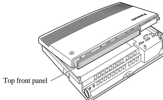
3. After cutting the areas, be sure to cut off any excess plastic in order to make the surface smooth. Please refer to installing the KX-TA62477.
