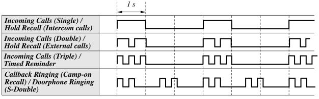
The Light Emitting Diode (LED) indicates the line conditions using lighting patterns.
