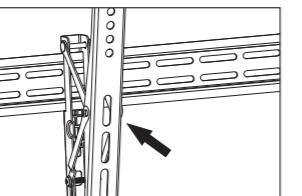
(2)Pull down two strings together to unlock the brackets from the wall plate,then you can take brackets down.
