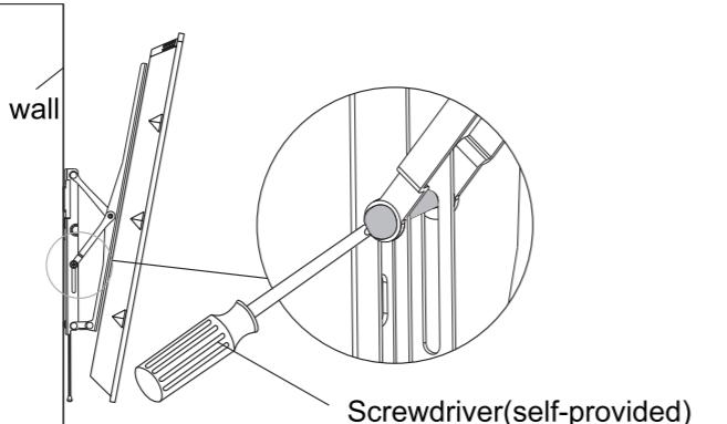
Your TV should adjust easily when moved, then stay in place. Adjust the screw clockwise with the screwdriver (as picture shown) if your TV naturally tilts up or down.
