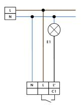
Parallel connection with 1-channel motion detectors
