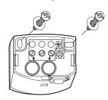
Mount the plug-in socket with two screws and the enclosed seal rings on a firm base. (Pay attention to inserting of the connection cable, see point 3.)
