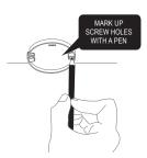
Use the mounting base ring to mark the screw holes on the ceiling or the wall.
