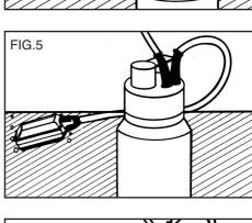
When the float switch reaches the minimum level it will automatically switch the pump off.
