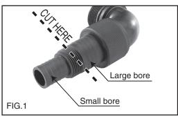
**NOTE:** The adaptor can now only be used with a large bore hose and cannot be used with a smaller bore hose.
