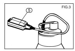
As the water level drops the float switch will fall with the water level.
