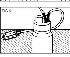
When the float switch reaches the minimum level it will automatically switch the pump off.
