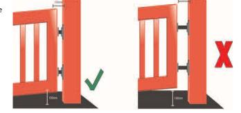
Figure 4 – avoiding gaps over 100mm
