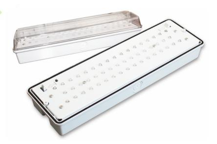
The 6W Emergency Bulkhead is an IP65 rated and has a polycarbonate base, a combined diffuser gear tray with quick release restraints and loop-in/loop-out terminals to allow quick and easy installation.
