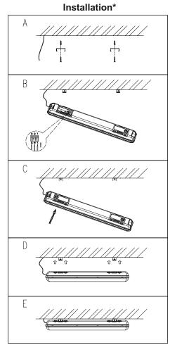
The fitting comes with both waterproof cable glands installed, one side has a silicone cover to ensure the IP65 rating. In order to utilize both connections, remove the blanking plate by unscrewing the cover.
