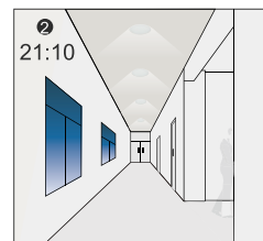
Light dimms to stand-by level after the hold time.
