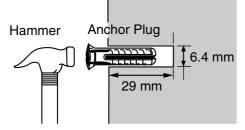
3. Fit the washers on the screws, and drive the screws into the anchor plugs.
