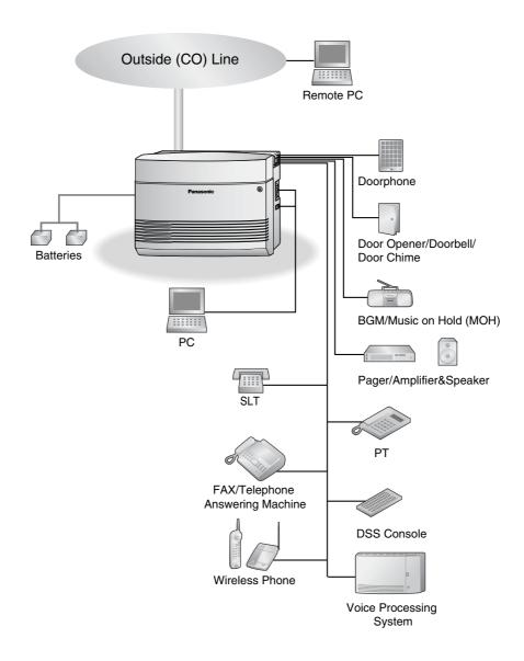
• Connect a display-equipped proprietary telephone (PT) to extension jack 01, as this extension is automatically designated as the manager extension.
