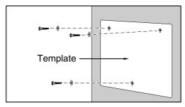
2. Drill holes in the wall as marked and fit the anchor plugs (not included) into the holes.
