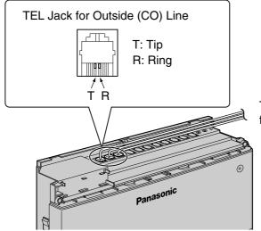
To Terminal Board or Modular Jacks from the Telephone Company
