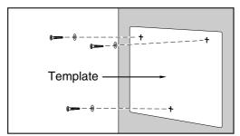
2. Fit the washers on the screws, and drive the screws into the wall.
