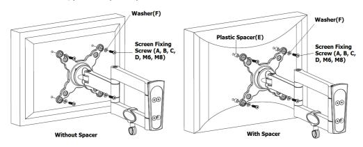
For VESA sizes bigger than 100x100, the supplied adaptors may be used. Attach the VESA extension arms as shown below using M5 12mm screws and nuts supplied.
