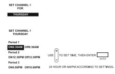
10.3 The OFF time will be highlighted for period 1. Use the advance buttons marked beside the + or – indicators to increase or decrease the value of the OFF time by 10 minute increments. Once the OFF time has been set press enter.
