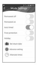
**Permanent OFF:** Output will remain off until auto is re-enabled by the user. In this mode, manual override is disabled and programmes will not run
