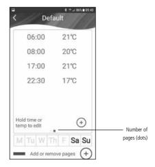
This shows the times when a temperature change has been programmed. The thermostat will maintain the programmed temperature until the next change.
