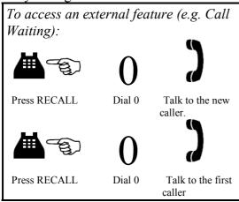
• If the Exchange Line Access Number Selection is assigned as "9", the external features access number becomes "9". For programming see page 26 of the installation manual
