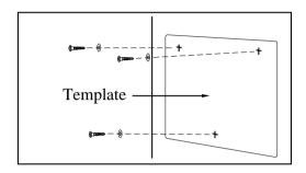
2. Install the screws (included) into the wall.
