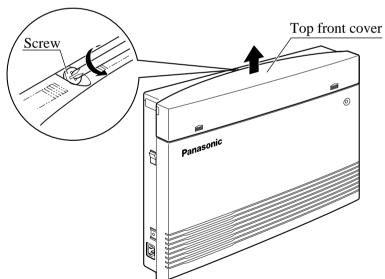
• The screw cannot be removed from the cover.
